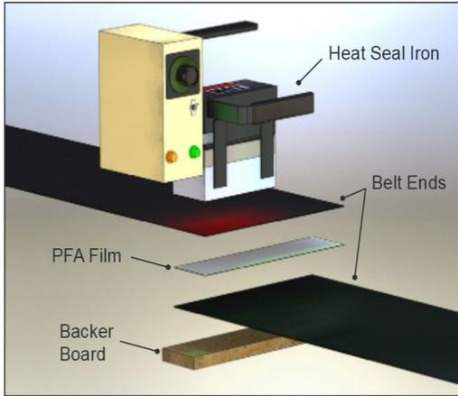
Upon purchase or rental of a FLEXXCEL Heat Seal Iron, U.S. Bellows will supply detailed Heat Seal Splice instructions specific to the belt material that you purchase. These instructions will include text, photos and drawings.
