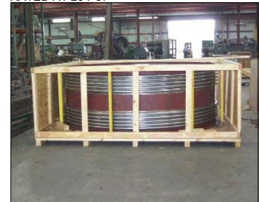
113" DIAMETER UNIVERSAL EXPANSION JOINT RATED AT 20 PSI
