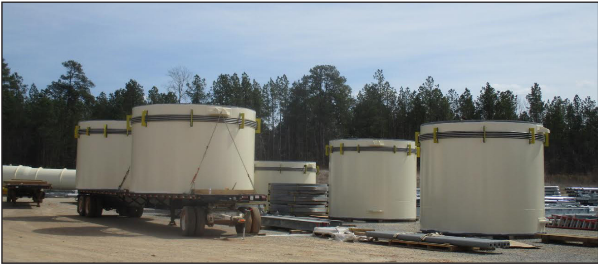
Figure 13 178" Diameter Tied Universal Expansion Joints On-Site
