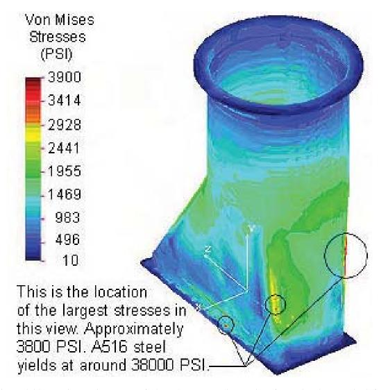
This model has an internal pressure of 18.7 PSI on every internal surface. The chart on the left of the model shows the stresses at every point in the model by a color coding system.
