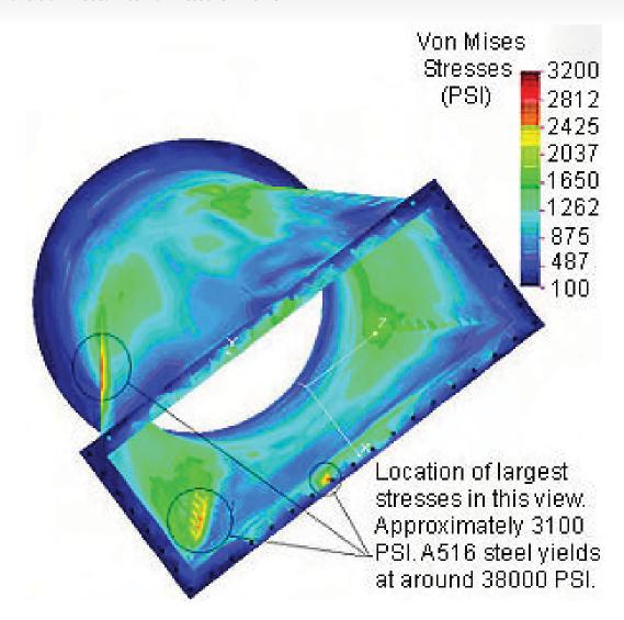
This model has an external pressure of 15 PSI on every external surface. The chart above shows the stresses at every point in the model by a color coding system.
