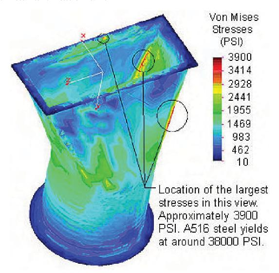
This model has an internal pressure of 18.7 PSI on every internal surface.
