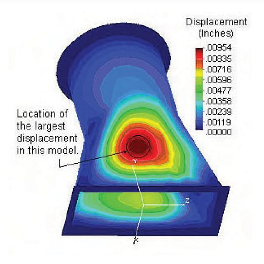
The chart above shows the displacement at every point in the model by a color coding system which represents inches of displacement.
