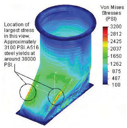
The chart above shows the stresses at every point in the model by a color coding system. This model has an external pressure of 15 PSI on every external surface.
