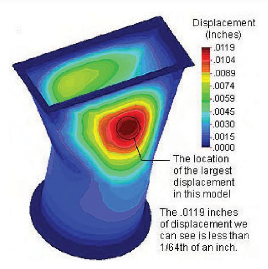
This model has an internal pressure of 18.7 PSI on every internal surface. The chart shows the displacement at every point in the model by a color coding system which represents inches of displacement.
